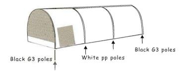
Insert the black G3 poles into the bottom pole sleeves of the two sides,insert the white PP poles into the two middle sleeves.
